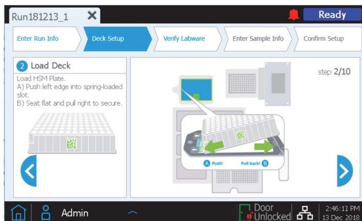
Figure 7. Step 2 of 10 of the Deck Setup screen of the Magnis NGS Prep System
