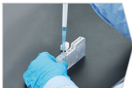
Load the sample into the iCassette
